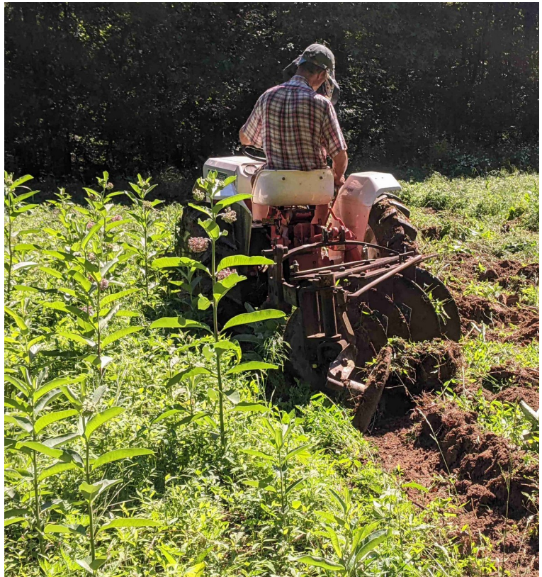
Disc tiller/ poly disc behind Sally. Much more fuel efficient than a plow. (Milkweed on the left to support Monarch butterflies.)
