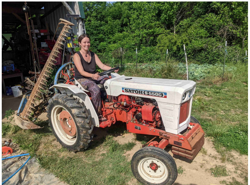
Chryssy (the person) driving Sally (the tractor). This mowing rig takes about 1/4 as much fuel as a bush hog.
