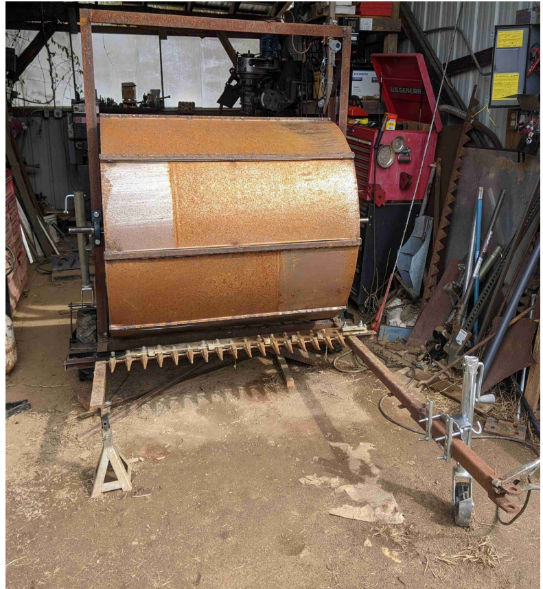
The Grain Goblin, the next generation simplified combine harvester, being assembled in our shop with our direct drive shop tools and solar powered welder.
