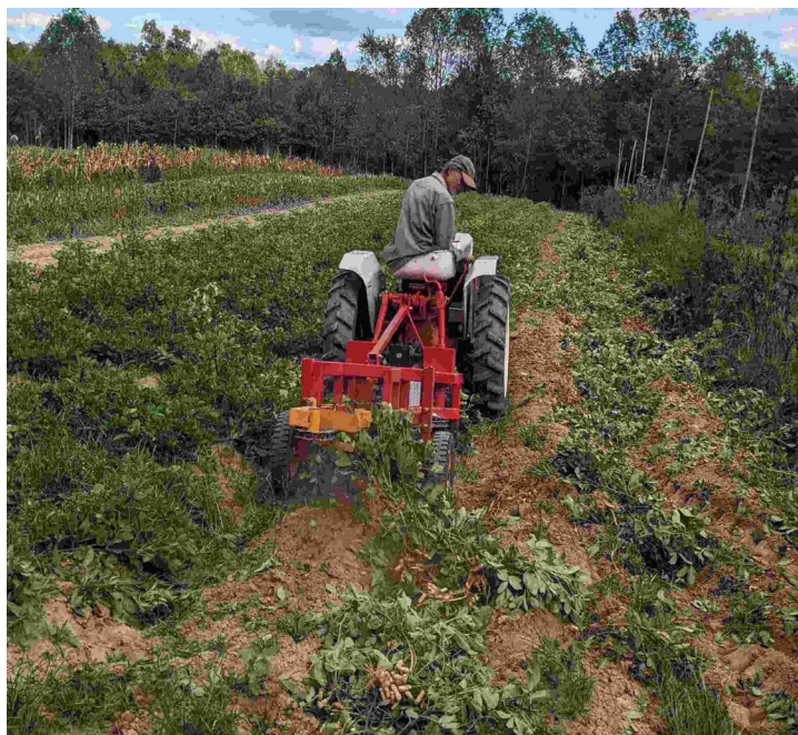
Digging peanuts with our new one-row peanut digger. Works great! We hope to be running that tractor on biogas soon.
