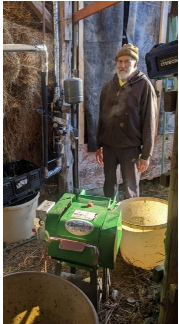
Otto has taken diligent care of Seymour, our biogas digester, with good results. The green device in the foreground is a silage chopper we brought in from China. It is very helpful in preparing organic materials for Seymour.
