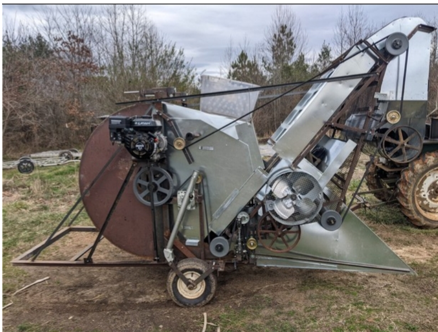
The Easy Reaper. Future Easy Reapers will look very similar, though the big round part on the left (the thresher) will likely get smaller.
