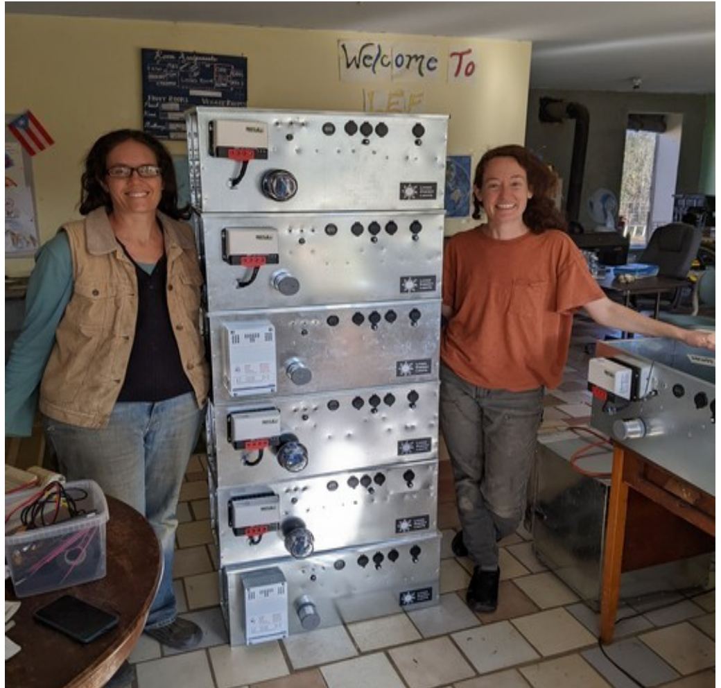
Nickel iron battery boxes built by Debbie and Carrie. These will last a long, long time.
