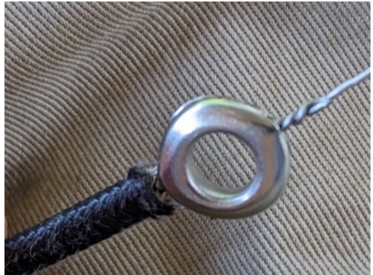
Nichrome wire riveted to high temperature wire. Nice to have a real machinist on our team.
