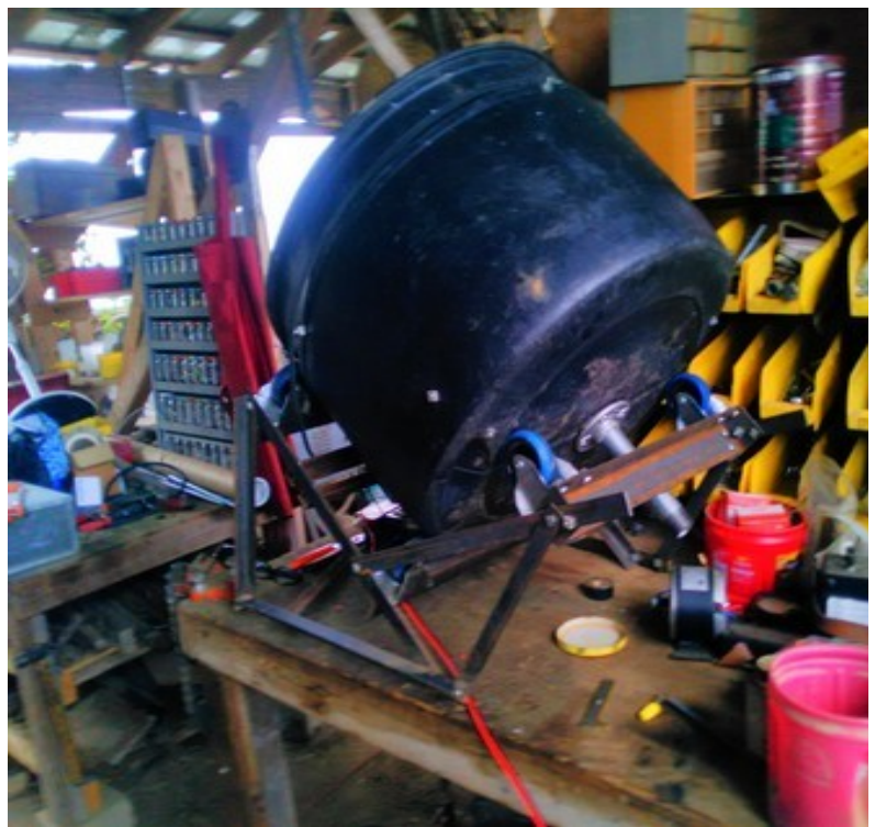
Prototype DC washing machine. Rotates on casters with an Archimedes Screw (spiral pipe) inside so it can drain without tilting.
