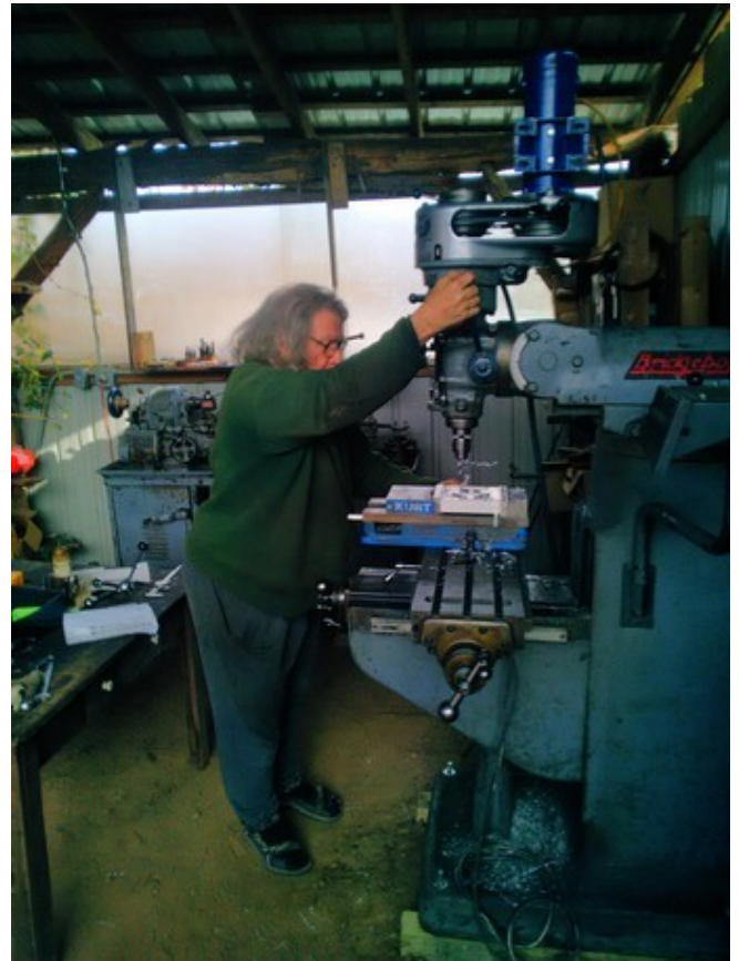
Kris running our new daylight drive powered milling machine at LEF.
