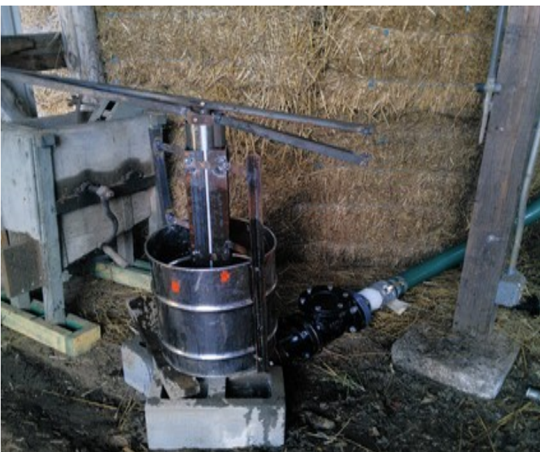
Our new biogas slurry pump for pushing organic material into our third generation digester. It is a big improvement over trying to push organic material in by hand.
