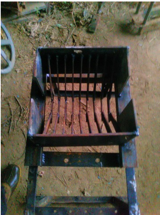
The shaft with blades drops into a welded box. Organic material is crushed and pushed through the slots.
