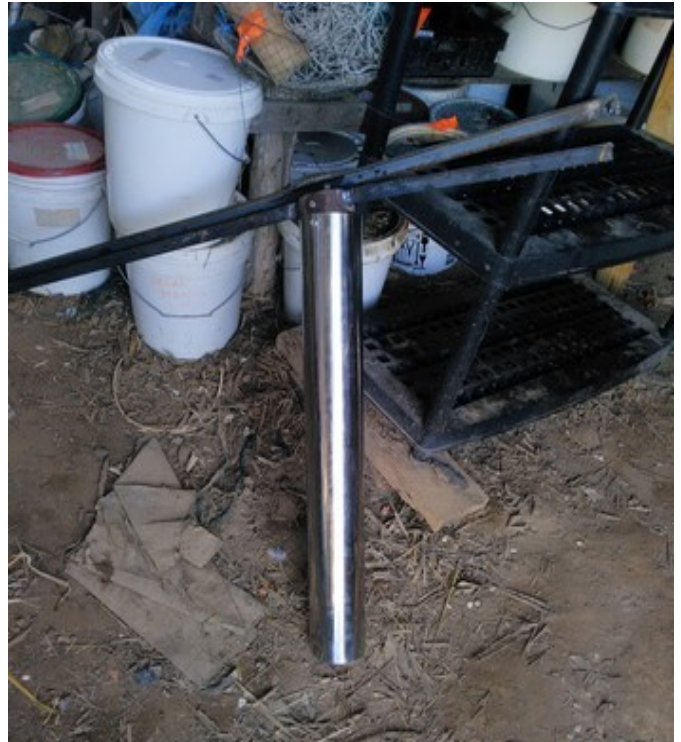
Sleeve and piston assembly for our new biogas slurry pump.
