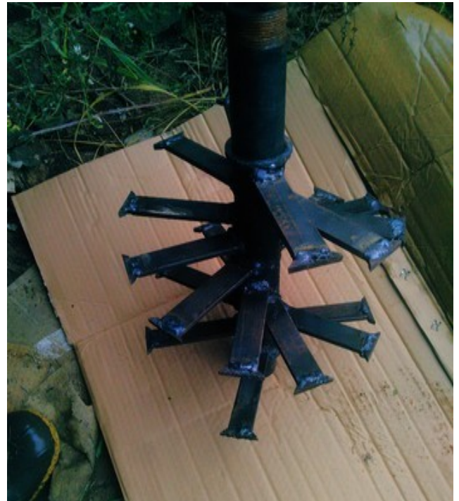
Our new biomass grinder has a spiral of heavy blades welded to a 1.25 inch black steel pipe.
