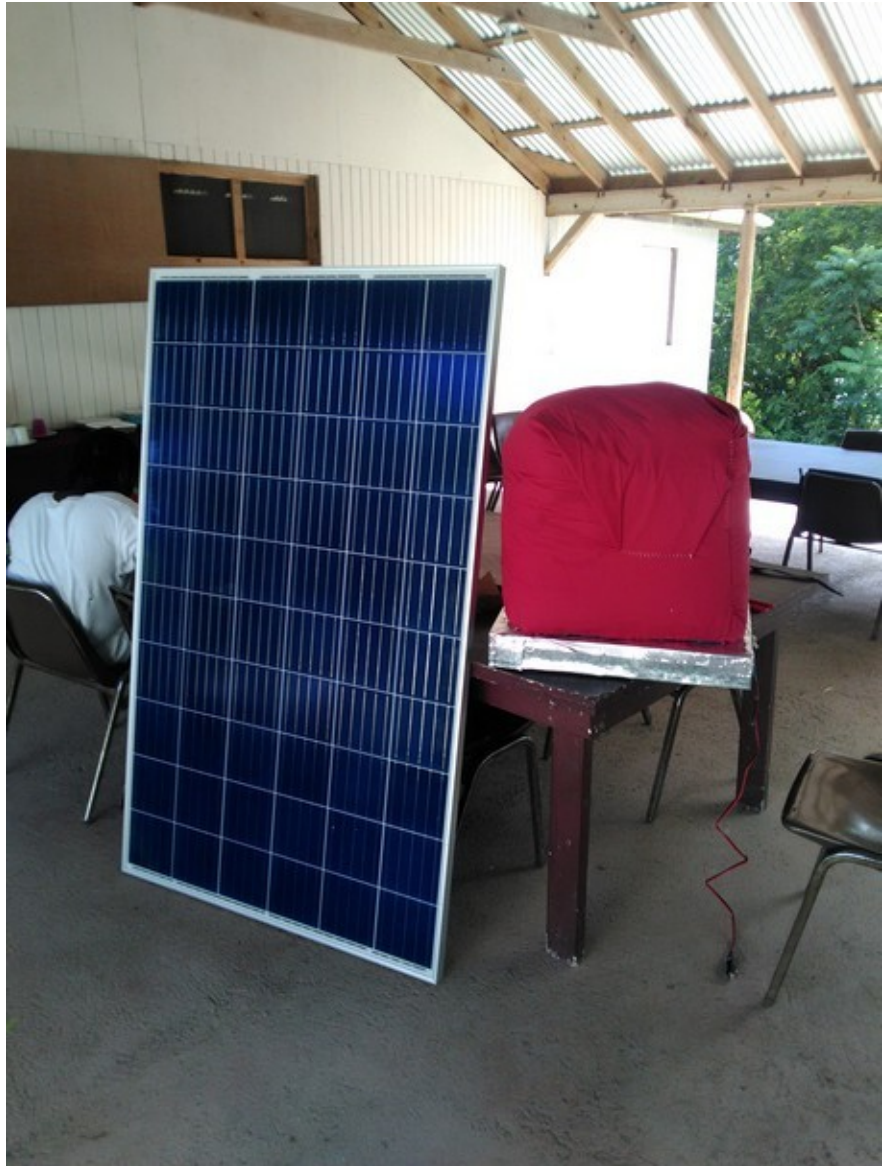
We built "Red Roxy" in Jamaica, placed here in an outdoor kitchen. At 300 watts, it will demonstrate a stronger cooker than our 100 watt Perl bucket cookers.
