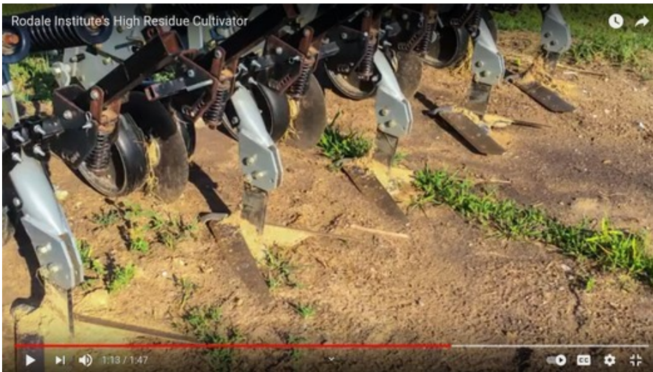
Screenshot from Rodale's youtube video about their high residue cultivator. We plan to use similar heavy steel sweeps to undercut cover crop so we can plant our no-till earlier.
