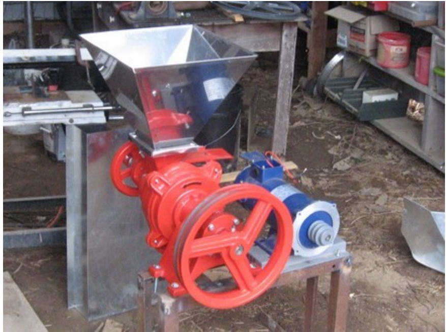
Breadfruit grinder, headed for Jamaica, daylight drive DC powered. No fossil fuel or industrial solar needed!
