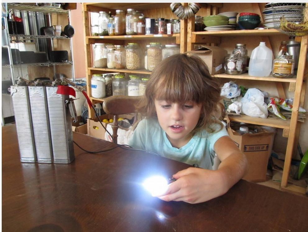
**1) Durable batteries.** The battery shown here works, and it's about 100 years old. It is a Nickel Iron (NiFe) battery. NiFes were produced by Thomas Edison in large numbers. They tolerate voltage swings and discharge depths that would destroy any other battery. Technology evolves toward profit, not function. NiFes were driven off the market because they are extremely durable, somewhat bulky batteries. Disposable batteries are more profitable.
