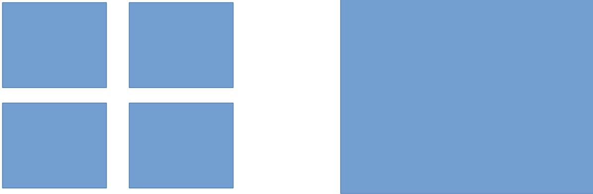
**7) Appropriate design** in cold climates means wrapping a well-insulated shell around shared structures rather than breaking down houses into “tiny houses.” The square on the right has as much area with half as much surface area as the squares on the left, thus representing the tradeoff between four small houses versus shared wall housing.
