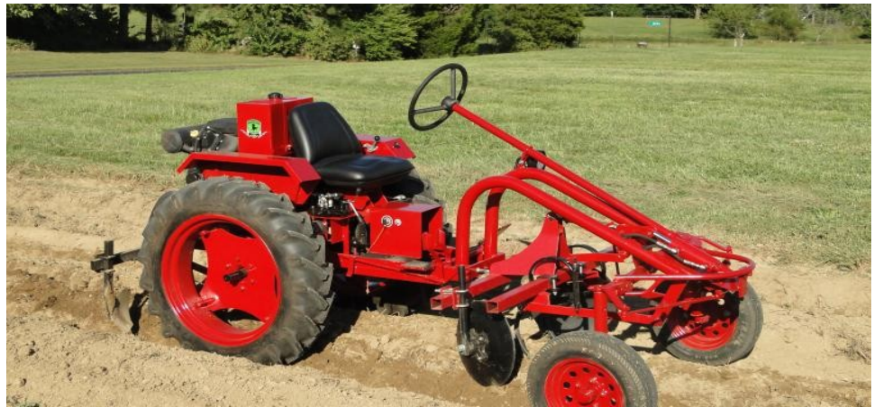
Oggun Tractor, similar to the classic Chalmers G and the Tuff-Bilt, but made to be locally produced.
