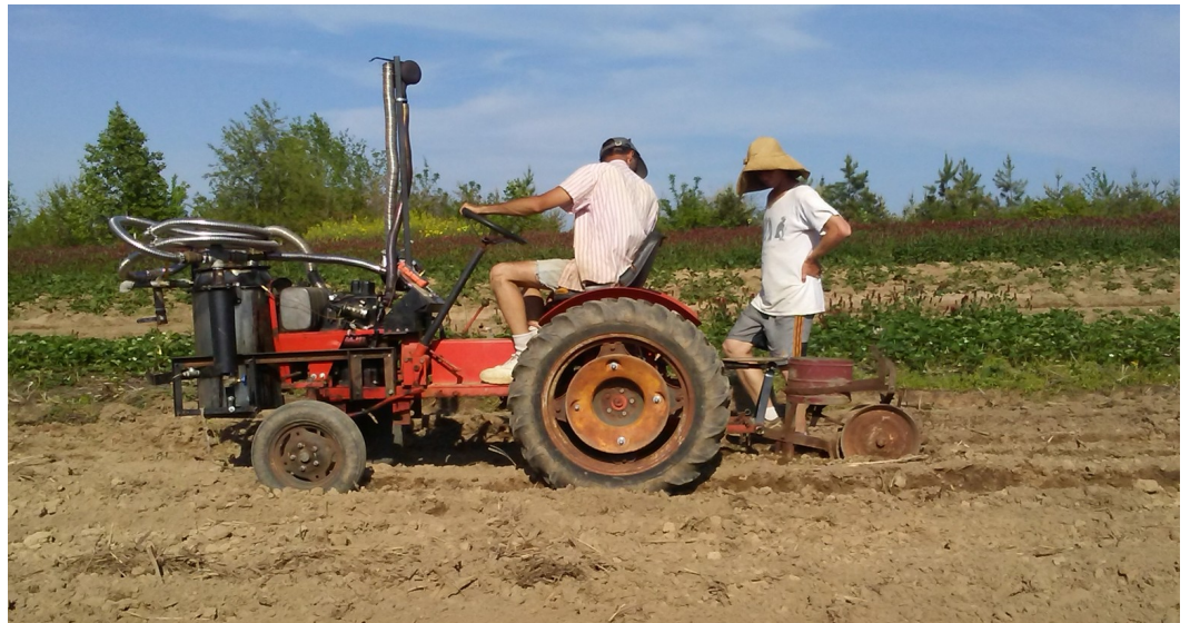
One-row Power King tractor running woodgas and pulling an old mule-drawn Cole planter
