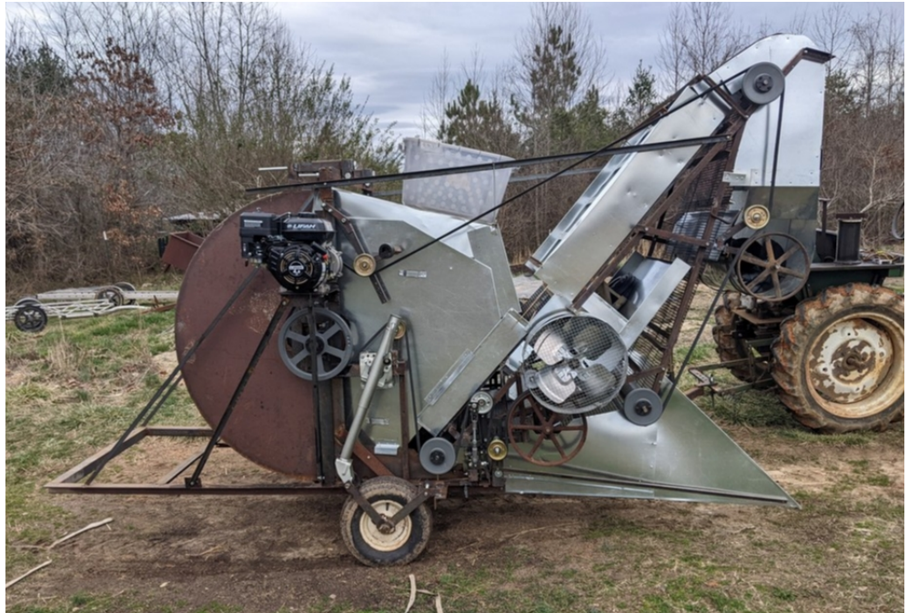
Simple Harvester, Prototype 3. With only one belt, it is by far the simplest combine harvester ever built as far as we know.
