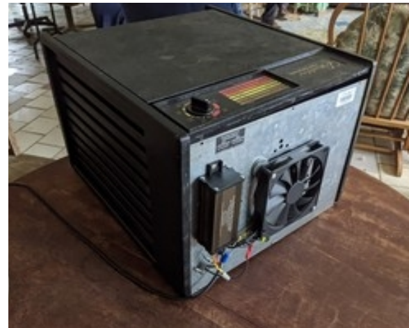
Food dehydrator converted to direct drive DC.
