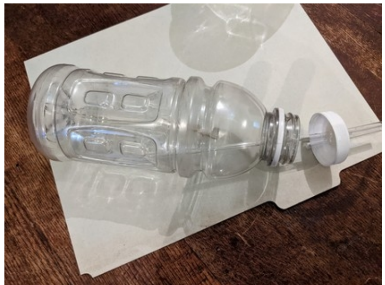
Battery waterer made from a juice bottle and some tubing. Works great!
