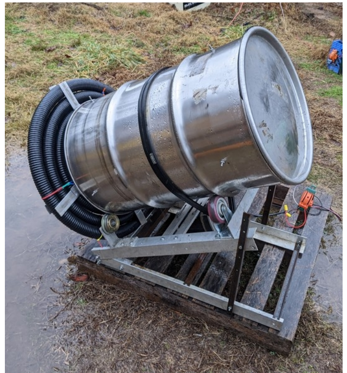
Direct drive, DC washing machine. Simple and effective.
