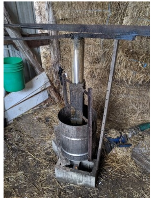
Biogas slurry pump, Piston sleeve and piston move independently.
