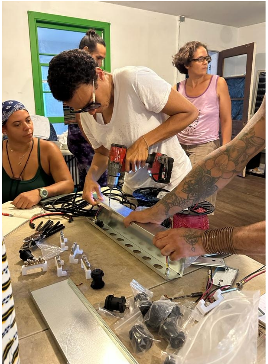
Millo working on a cigarette lighter plug strip for low voltage charging and appliances.
