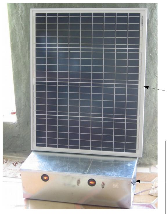
LELCS with PV panel. Note, LELCS have a charge controller built into the box. These controllers are small, inexpensive circuits that can handle a maximum 50 watt PV panel. To use a LELCS with a panel larger than 50 watts requires the use of a different charge controller.
