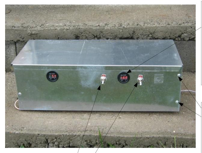
Voltmeter -- a normal LECLS box has only one voltmeter. We use a DC voltmeter, ebay item no. 283351933785 This voltmeter fits a 3/4 inch knockout hole made by the large lever punch specified later. Items can be found on ebay by searching with the item number.
