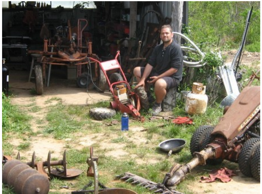
Dan, a skilled mechanic, stayed with us for a while and helped. The Gravelly sickle bar mower in the foreground use a lot less energy in mowing than a regular mower, and is one tough machine.
