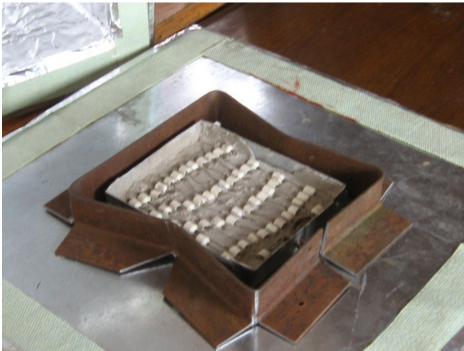
This is a radiant burner, 48 volt, 330 (or more) watts. It has a metal support around it to hold up a large pot (so the pot does not sit right on top of the burner.) A burner this size (it has 64 inches of nichrome wire) could not be built as a brick burner.
