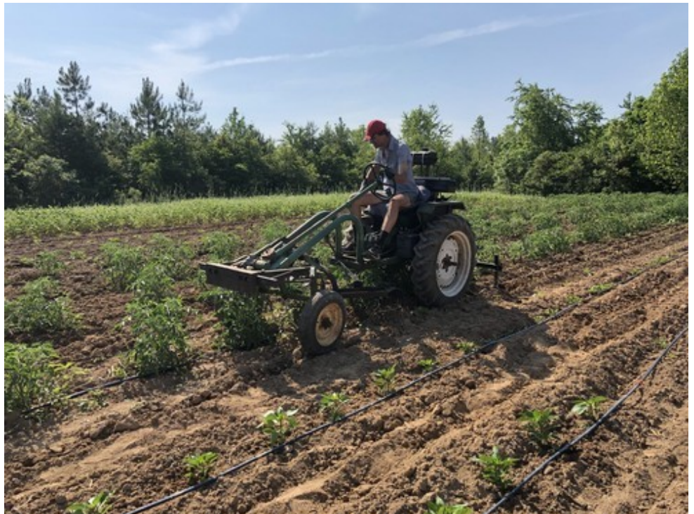
Running a Tuff Bilt tractor on turpentine from pine sap. Turpentine is much, much easier to use than woodgas, which we had tried to use previously.
