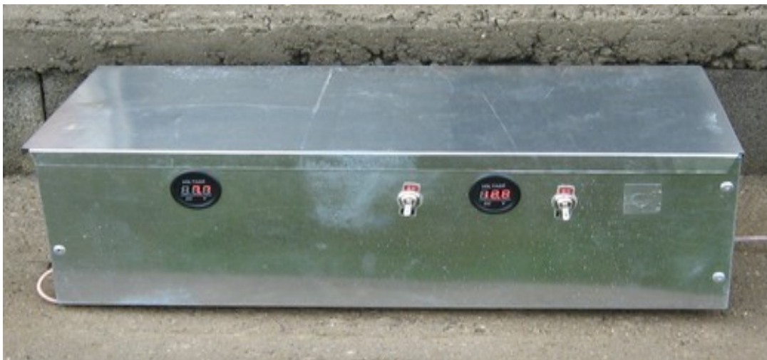
LELCS are enclosed in a custom made, durable metal box.
