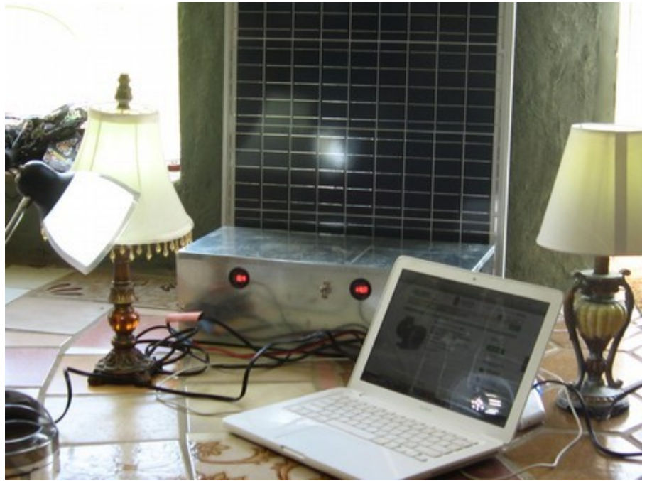
New LELCS kit running 3 lamps, a laptop, and a smart phone.
