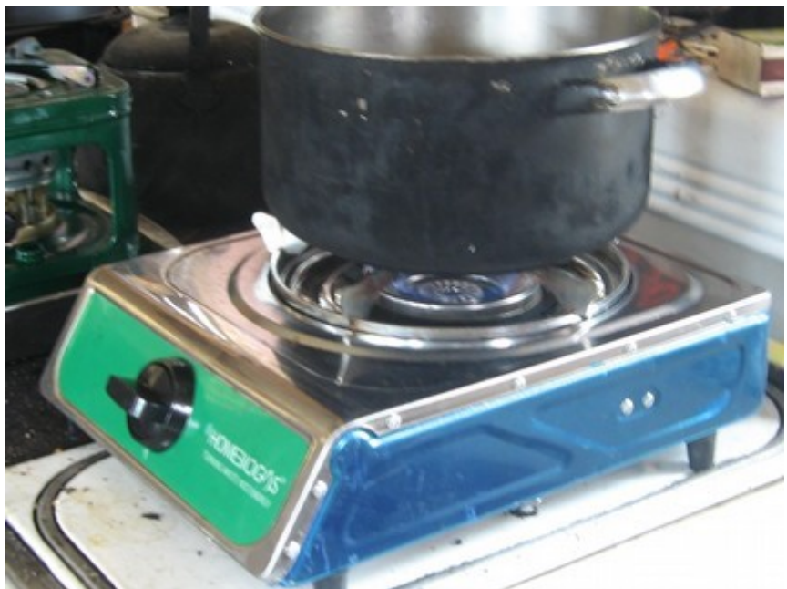
Biogas burner, excellent heat output, tolerates variations in gas quality and pressure very well.
