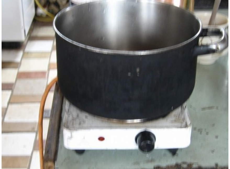
220 volt AC hotplate running 180 volt DC daylight drive power. We bypass internal switches and use external butterfly switches.
