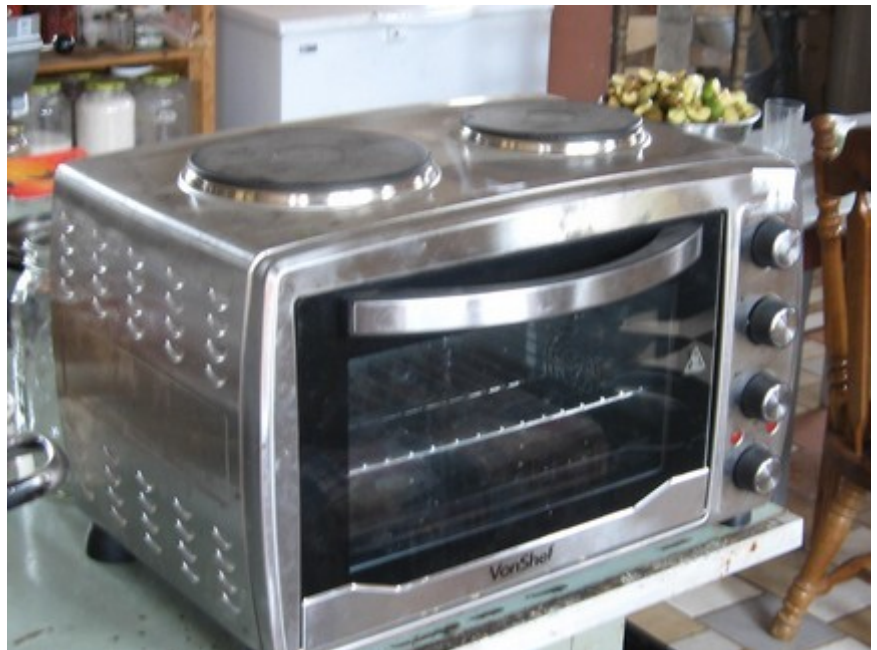
220 volt AC oven with hotplates running off of 180 volt DC daylight drive power. Bakes great! Again, internal switches bypassed.
