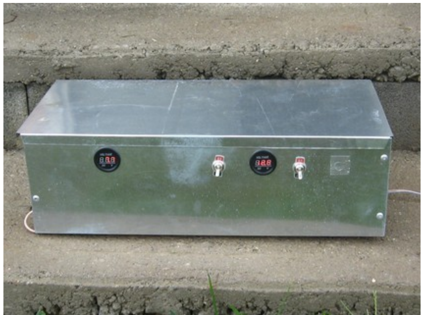
New LELCS metal enclosure. Takes some time to build the box, but it's better than the plastic toolboxes. Round meters and switches can be installed quickly using standardized punches.
