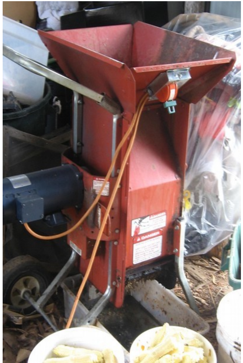
The explozerator -- yard shredder equipped with nice, heavy duty industrial DC motor. A little spooky how quickly this thing obliterates organic material.
