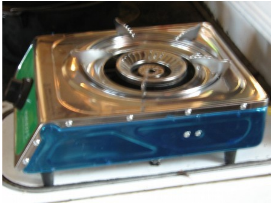
Biogas burner. We have never been able to get biogas to burn well through a conventional gas burner -- not sure why.
