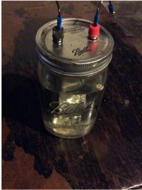
Homemade NiFe battery at LEF. Low power density is fine for residential use.
