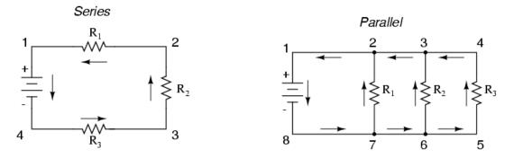
Understanding series and parallel circuits (illustrated above) is important. The symbol on the left of each drawing is the power source. The "Rs" are resistors, or devices that use electricity. The terms series and parallel apply to both energy production circuits (several solar panels) or to energy using circuits (the wiring in your house.)
