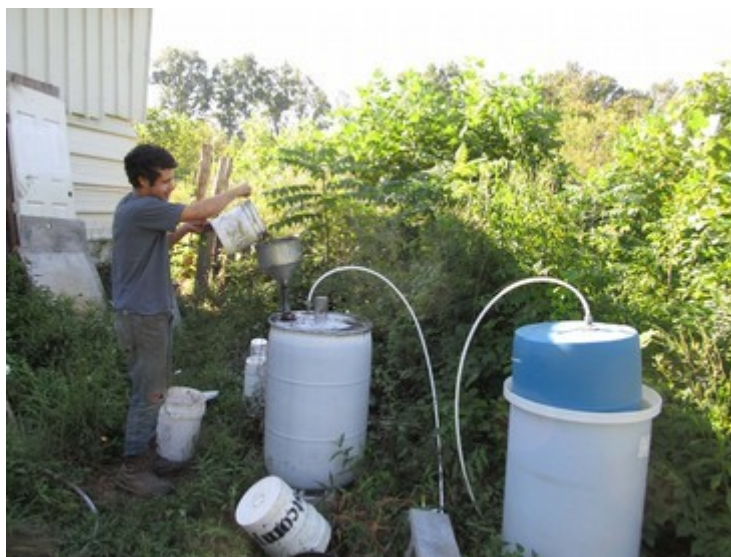
LEF's biogas unit from about 5 years ago. Gas production was meager, but we were new to the technology. We are focused on making a better biogas system now.
