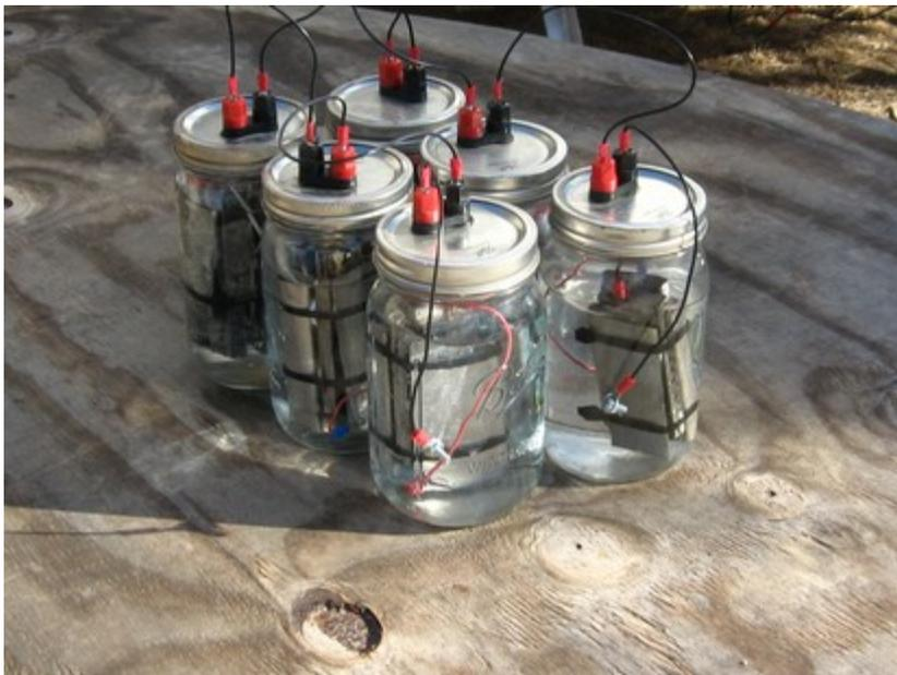
*Homemade nickel iron batteries, but they don't hold power very well (yet).*
