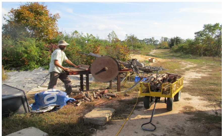
Cutting stove wood with solar power straight from our PV panels, MUCH faster than a hand saw, and with no batteries or inverters.
