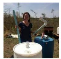
Carrie shows the two plastic barrels and PVC plumbing to be used in our biogas digester.
