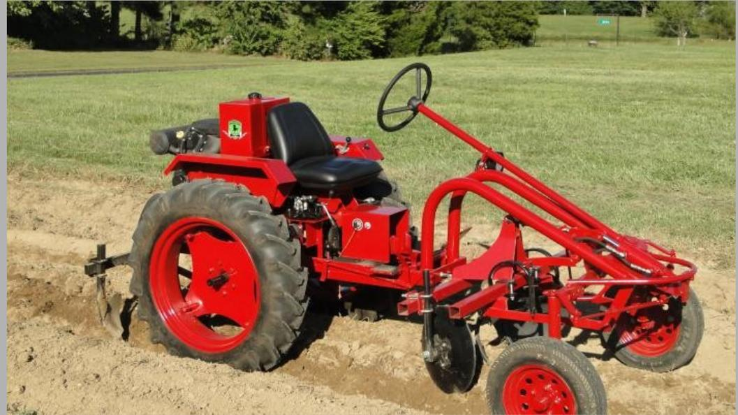
This is an Oggun tractor. Notice the engine is mounted in the rear. This is a modern, well designed agricultural tractor based on similar historical designs. Incidentally, the company was founded with the mission of providing inexpensive, easily constructed and repaired tractors for small farmers around the world.
