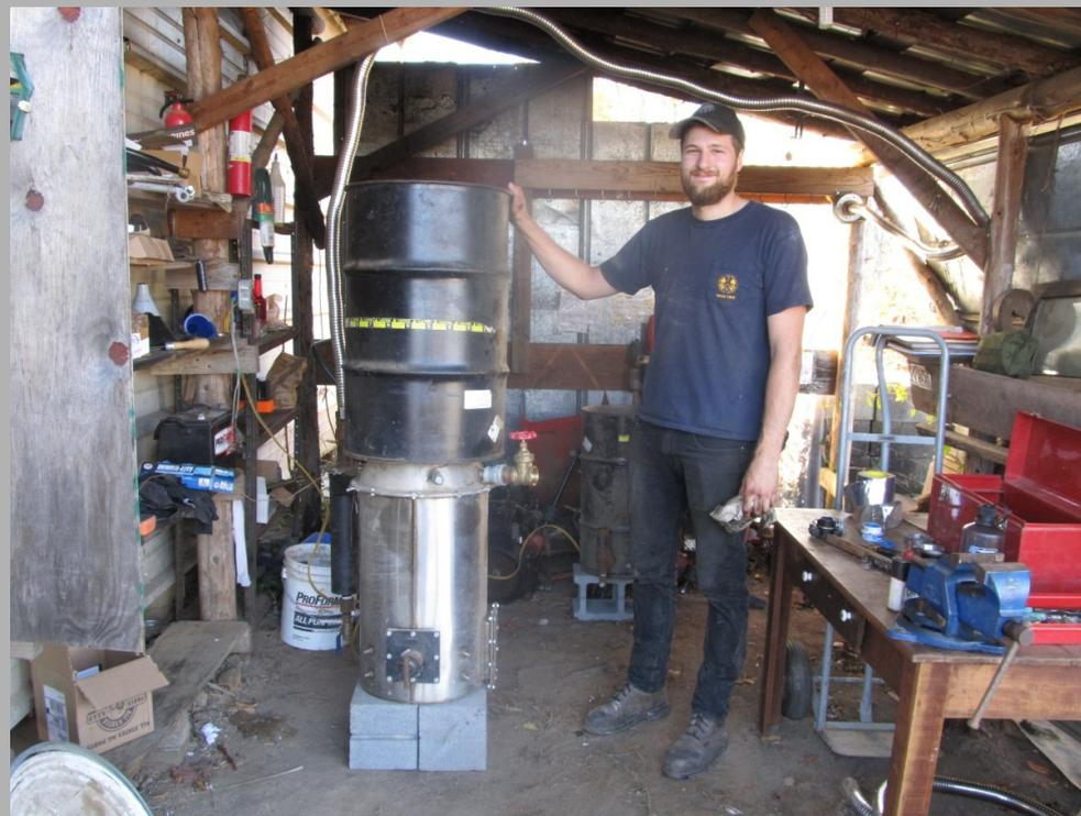
This gasifier was intended to be a stationary unit, but we modified it for use on a tractor.
