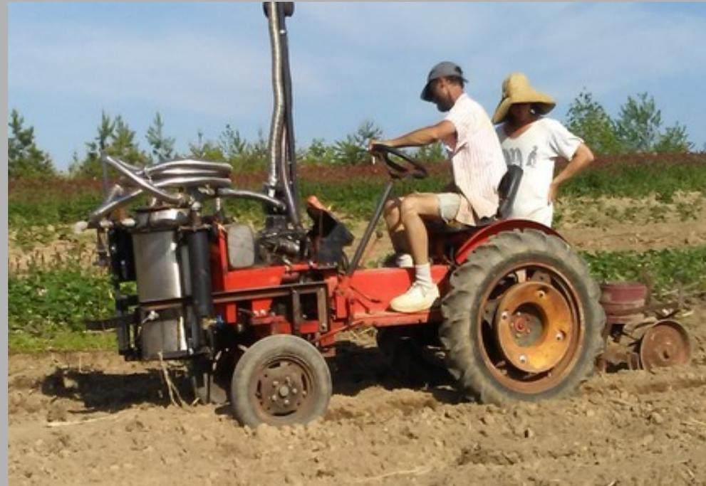
We repaired the gasifier and transferred it to this tractor, which has 1/2 the horsepower of the Ford where we used the gasifier previously. The engine on this tractor is in poor condition, and it is a more modern, higher speed, higher compression engine. The gasifier and the tractor worked, but not well.
