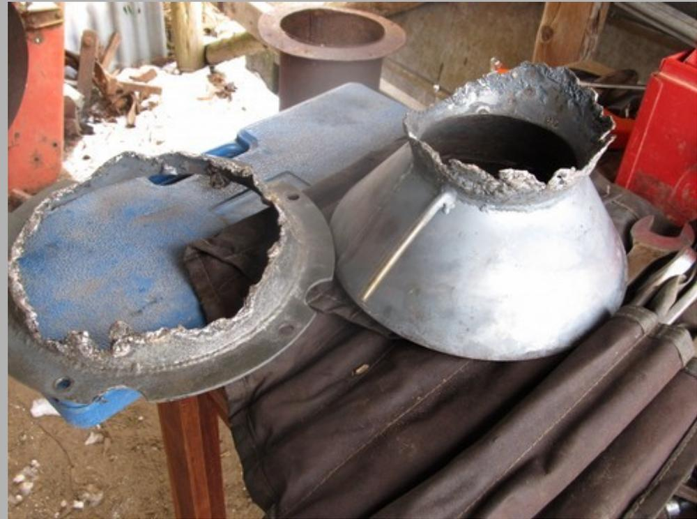
Every wood gasifier has an hourglass shaped reactor at its core. The shape and size of this reactor core has to be correct for the type of fuel and the size of the engine. And when you have a reactor that is too small for your engine? Sadly, it melts from excess heat.
