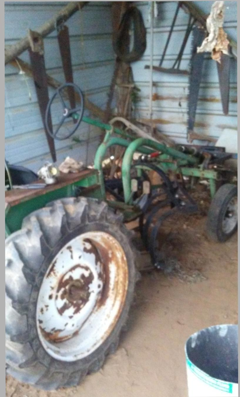
Rear-engine Tuff Bilt tractor at LEF. Engine is being swapped to a low compression engine that we can run on woodgas or turpentine.
