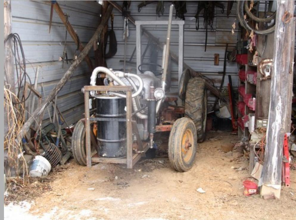
This is our wood gasification unit on the front of a 1961 Ford tractor. We ran this tractor on woodgas for a while, but the gasifier was too small (even though the tractor only has 35 horsepower).
