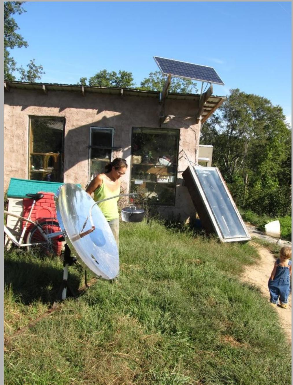
From the early days of LEF. We have used our parabolic cooker a lot. Batch water heater works great for 3 seasons. One small PV panel provided electricity.
